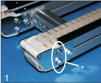
Remove two screws (\*) and loosen the third one.
