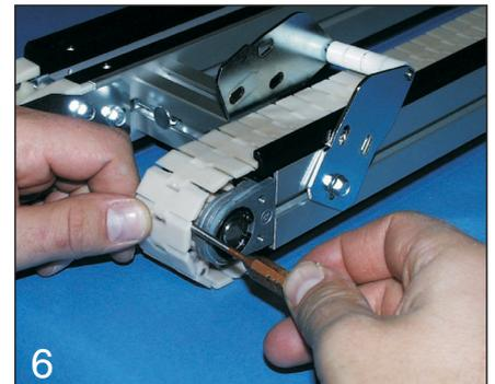
To re-assemble the chain, press the steel pin back to join the links.
