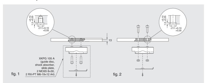
The guide disc can be mounted on to the pallet base in two ways.
