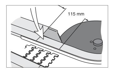
If the length of the pallet exceeds 300 mm, a 115 mm piece of XKRS guide rail has to be inserted before and after each wheel bend. This is to prevent the pallet from getting caught by the guide rail in the bend.
