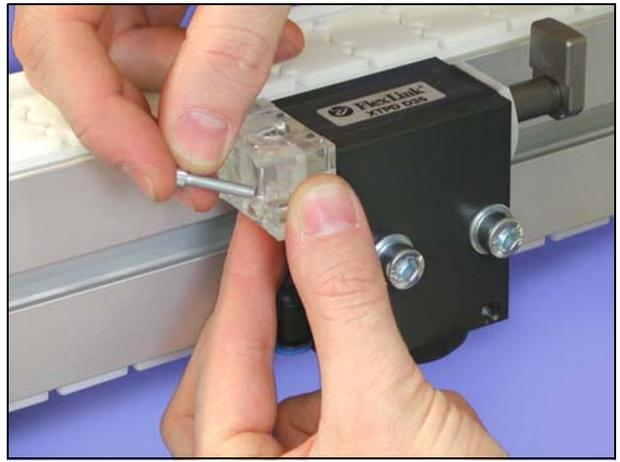
4 Fit the sensor to the sensor bracket.
