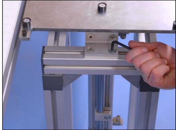
9 Adjust the support, unit and/or the conveyor so that the lift and locate device is positioned correctly.
