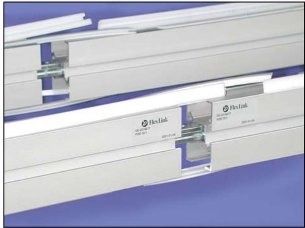
5 Tighten the screws. Use the 4 mm allen key.
