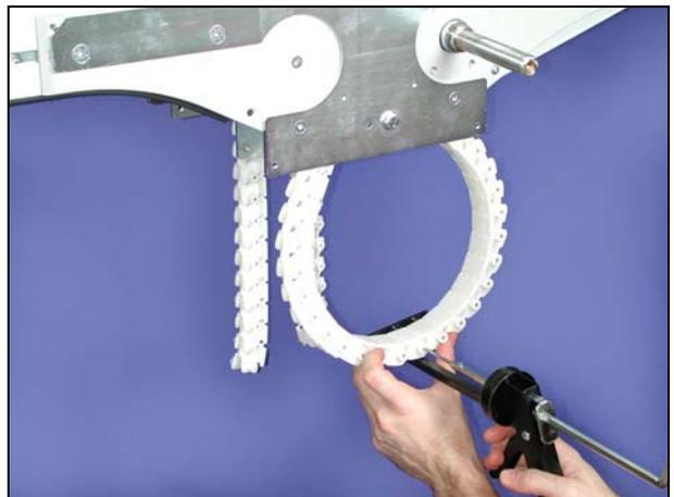
11 Make sure that the pin snaps in to the correct position (centered).
