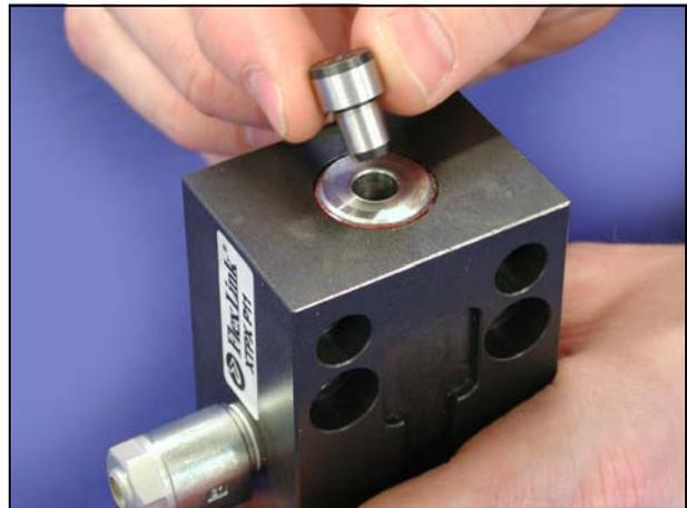
2 Use a soft faced hammer and hit the pin carefully until it reaches the end position.
