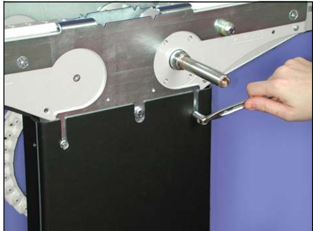
14 Fit the plastic sleeve on the drive shaft.
