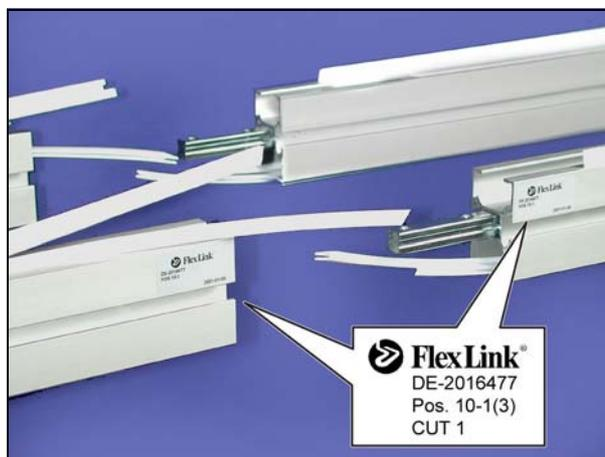
4 Make sure that the conveyor section ends fit together properly.
