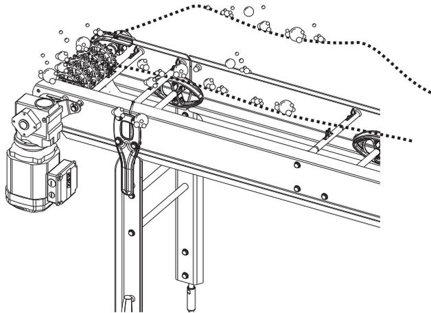
The disinfection should not be applied with pressure but with a specially nozzle for spreading disinfectant solution on all surfaces. Leave on for typically 10-15 min (follow instruction from disinfectant solution supplier).
