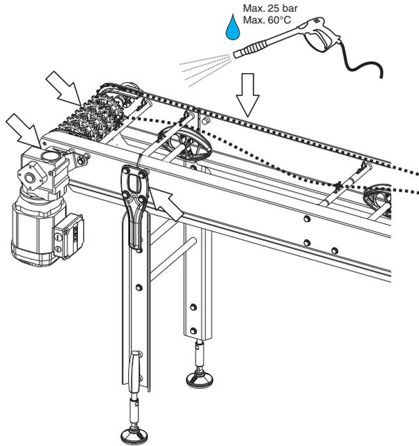
In pre-rinsing, soil is rinsed off or detached using warm water (up to 60°C) at low pressure (max 25 bar).
