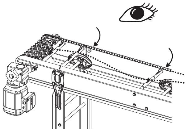
The final cleaning and disinfection result is checked before the production is started up again. An appropriate culturing method in accordance to the food producer internal control system should be used (swab, contact plate).
