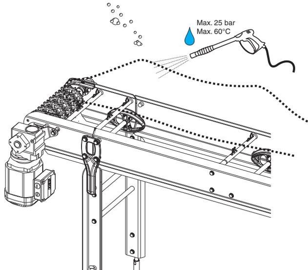
No cleaning chemicals residues should be left on surfaces. Therefore the chemicals should be rinsed off with lukewarm potable water. Thereafter the equipment should be left to dry.
