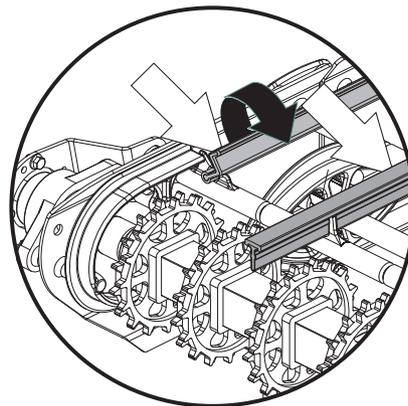
Idler end wheels have an open design and can easily be moved sideways in order to facilitate cleaning of the shaft. When conveyor belt is removed also drive sprockets can be moved sideways.
