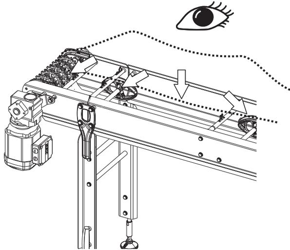
The cleaning result is checked visually and by hands to feel that the soil has been removed. Here an appropriate method e.g. ATP-kit or protein based kit can also be used.
