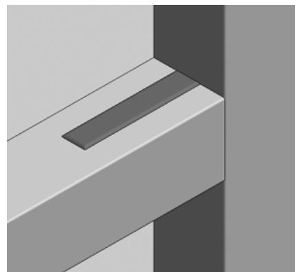
Caps for covering connecting elements to provide an aesthetically pleasing finish.
