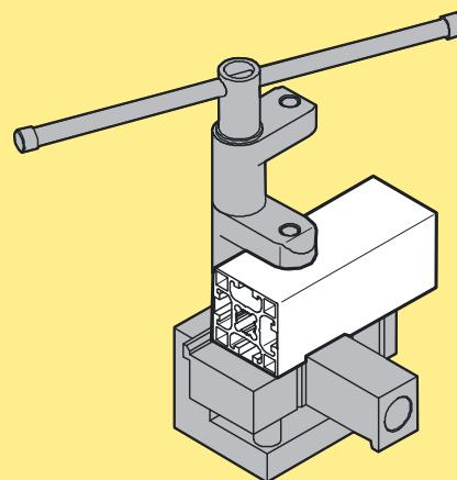
Punching tool, to open closed T-slots
