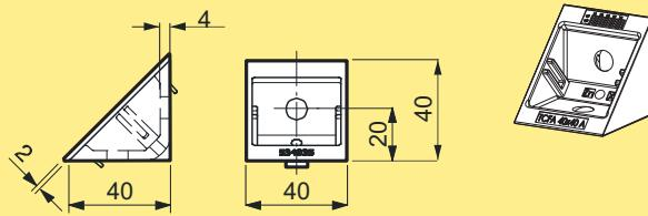
Angle bracket, 40x40, die-cast\* **TCFA 40x40 AB\***
