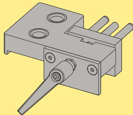
Drill fixture, central joints-
