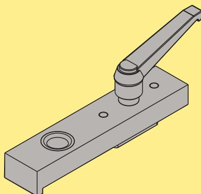
Drill fixture, central joints
