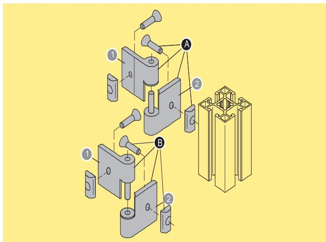
A Hinge LS/ M6x12 countersunk-head screw/ M6 T-slot nut
