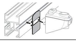
**Tip:** Mount one complete guide rail bracket kit on the beam for correct measurements. Assemble the rest of the kits on a mounting table by copying the first kit. Click kits onto beam when complete.
