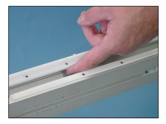
12 When you reach the end, cut the slide rail so that there is a 4 mm distance to the next piece of slide rail.
