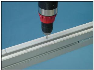
10 Fit the rivets in the holes and press them together with the rivet tool.
