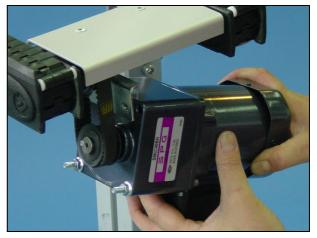
5 Fit the screws holding the motor.
