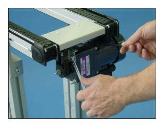
4 Remove the screws holding the motor. Remove the old motor and fit the new motor.
