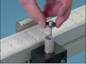
5 Place washer (D) on the pipe (B) and fit the screw (A) and washer (C).
