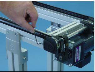
5 Remove the screws (4×) on the inner side of the drive unit, use the 8 mm box wrench.
