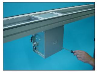
2 Remove the screws (2x) holding the motor, use the 5 mm Allen key and the 10 mm box wrench.
