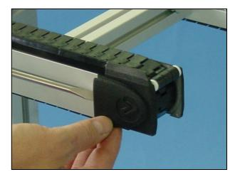
2 Use the 3 mm Allen key to loosen the screws on the idler end.
