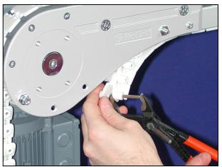
11 Join the chain endings. Make sure that the joint ball has not been removed and re-assembled upside down.
