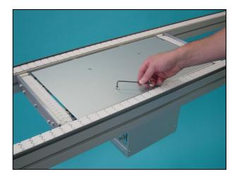
2 Remove the screws (2×) on the transfer unit bracket. Use the 5 mm Allen key.
