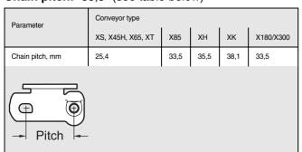
**Actual CC distance (mm):** The selected CC distance will be round off to the closest value which matches the chain pitch.
