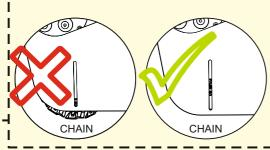
The conveyor chain must be maintained during system lifetime. If the conveyor chain is too long,it must be shortened.
