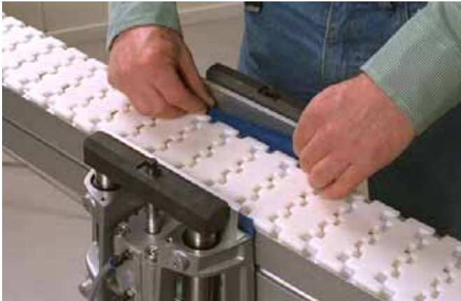
14 Place two distance pieces (2,5 mm thick) between the locating station and the conveyor beam, one on each side of the beam, to keep the locating station centered.
