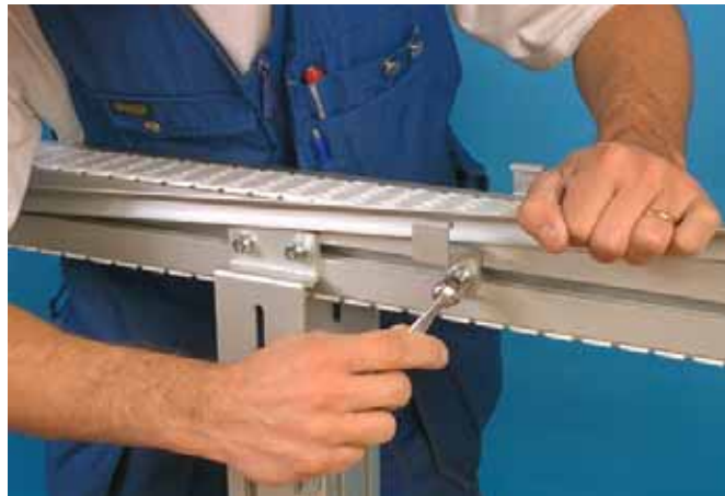
Angle plates and guide rail brackets (48x30) for the XL conveyor system.
