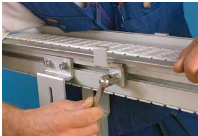
Angle plates and guide rail brackets (49x42) for the XM and XH conveyor systems.
