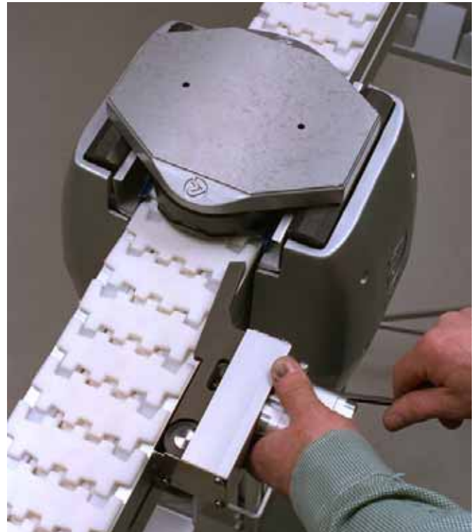
18 Position the pallet stop by placing a pallet onto the locating station. Then tighten the pallet stop 0,5–1,0 mm in front of the pallet (see drawing).
