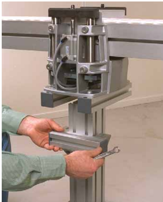
12 Position the locating station in the correct position on the conveyor beam. Raise the lower pair of beams so that they meet the upper beam pair.
