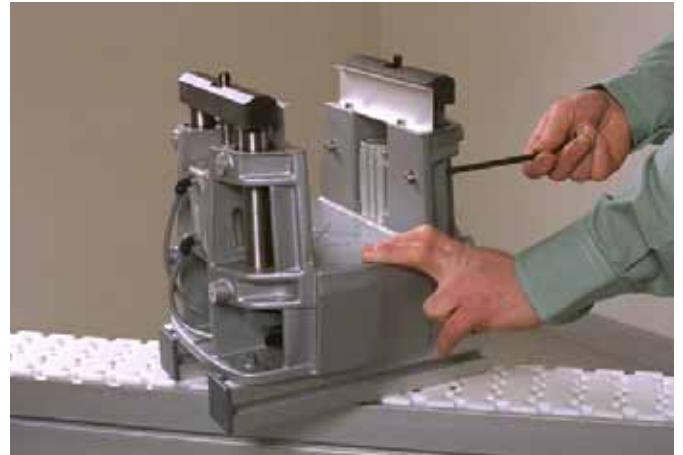
8 Tighten the guide pins on one side. Loosen the other pair.
