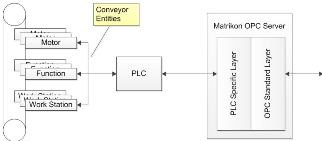
Within the PLC a segment of memory is used to convey messages to and from the MES solution via the Matrikon OPC Server. This segment of memory is sub-divided into a number of tags, each of which shall be used to convey a message in one direction or the other, but not both.
