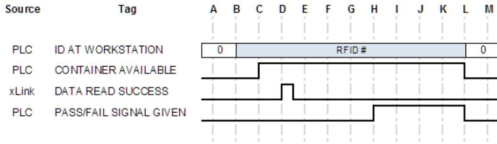
In those configurations where the Pass/Fail is set by the Mini Adapter the sequence of events is modified to include one extra communication so the mini adapter tells the PLC the status to report back to the mini adapter:
