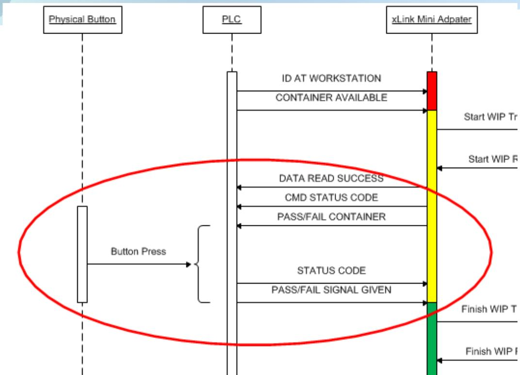
If the Release Button Required status (HS\_WS\_STATUS[Z].6) value is set low then logic within the PLC shall allow the issuing of a Pass/Fail Signal Given without any button press.
