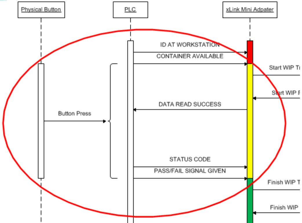
Further, in situations where the status of the PASS / FAIL is determined by Youtilize® (and not by the PLC) the PLC shall ensure the physical button is only enabled when the PASS / FAIL CONTAINER message has been received, and is disabled as soon as the PASS / FAIL SIGNAL GIVEN message is issued.
