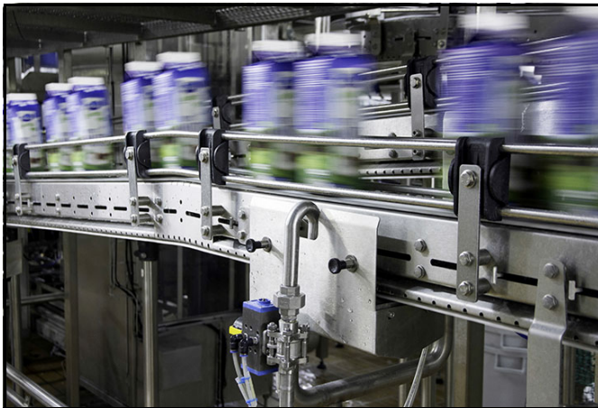
Milk packaging line with Clean-in-Place
