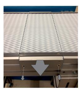
2. Insert the belt from the top: insert the front of the belt pointing towards the End drive unit.
