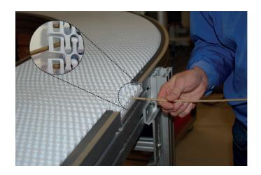
5. Press the rod into the belt until it "snaps" in place.
