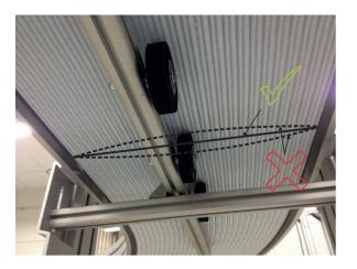
3. Wheels of the profile should be in line with belt underside, to high they will create a convex shape.
