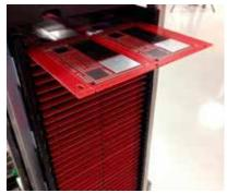
The PCB product line incorporates modular stand-alone units with on-board control, that are truly independent from other modules in the system. Each module is able to be linked to other modules in the system by utilizing their up line and down line SMEMA communication. The modules can also be linked to a higher level monitoring or routing system by utilizing a host control system.
