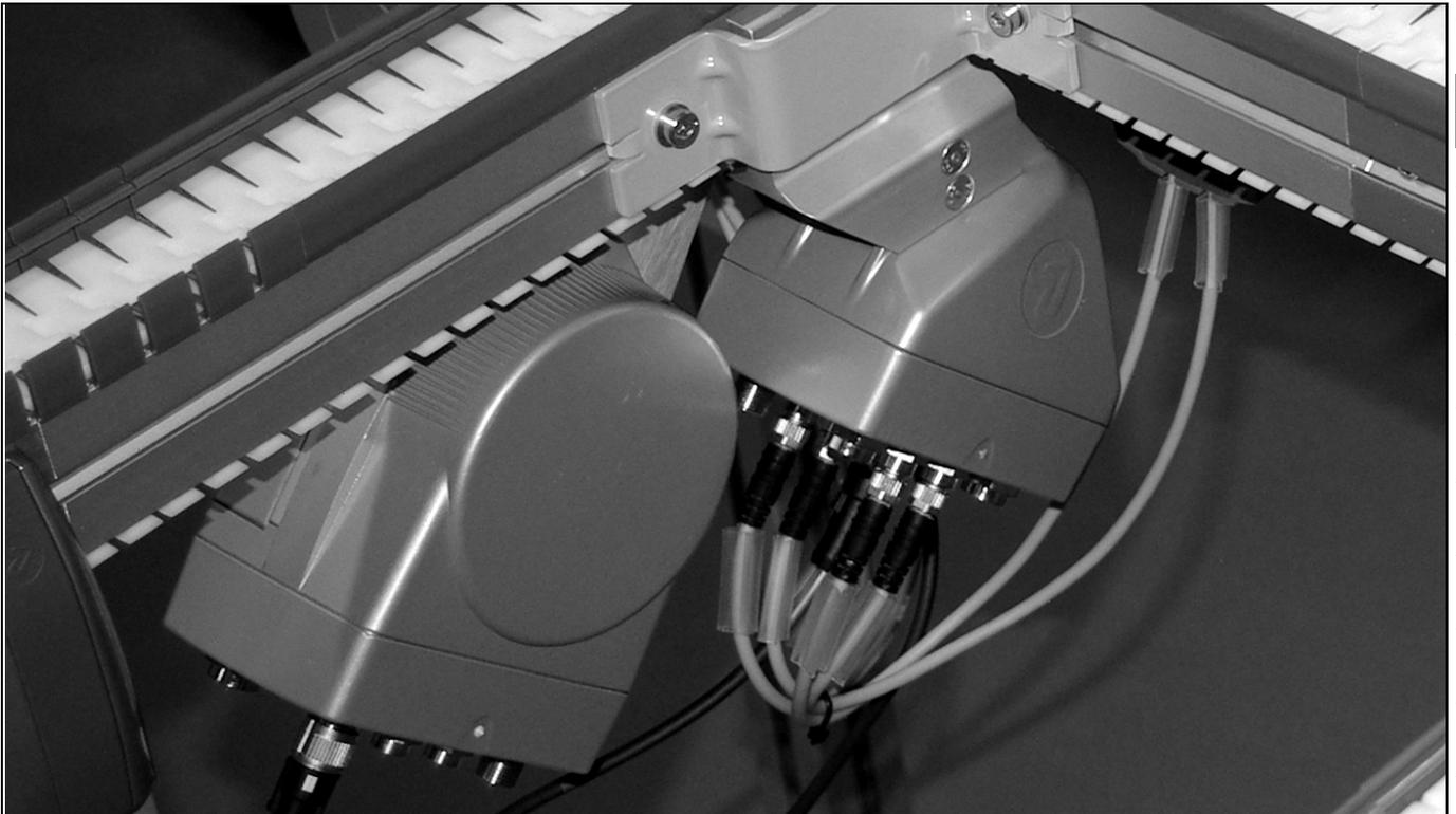
The control system for the platforms X45e is structured in an object oriented way. All puck function motors in the platform have embedded control units and local sensors are connected directly to each motor unit. This layout gives a big advantage regarding software developing, electrical design and electrical installation.
