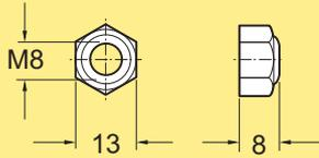
Locking nut M8 for T-bolt
