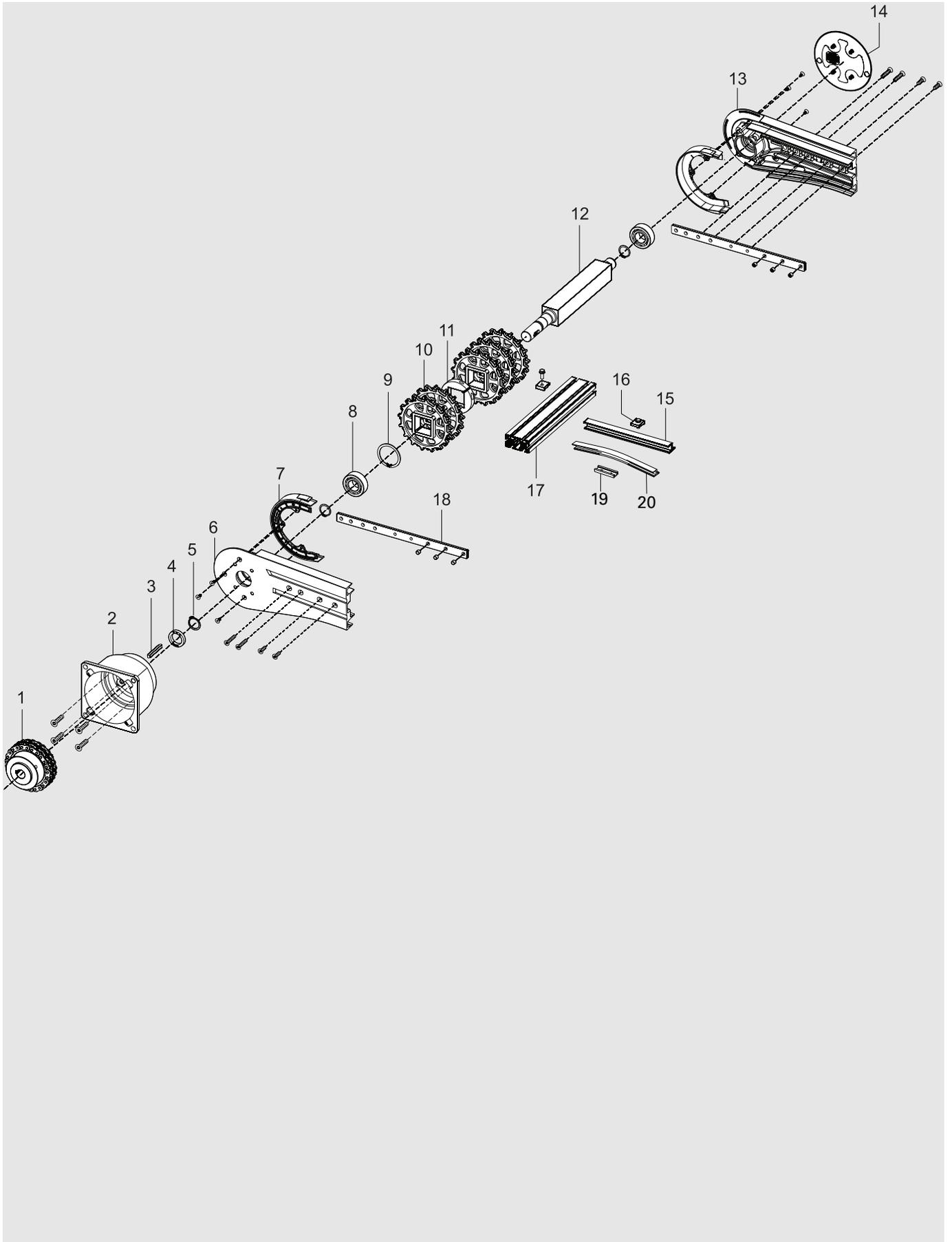
**End drive units, direct drive with slip clutch**
