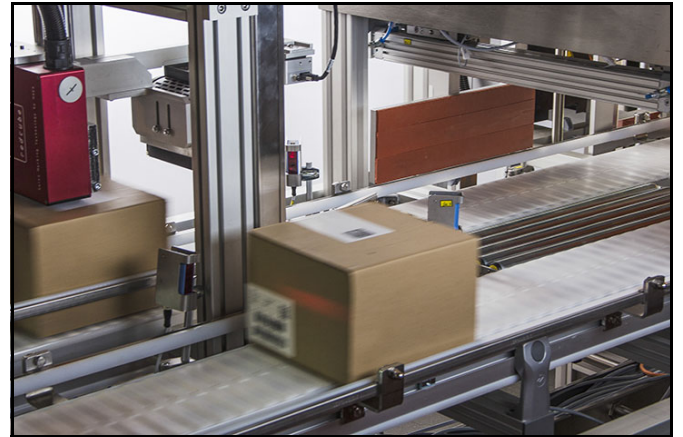
Advanced carton box handling with track and trace
