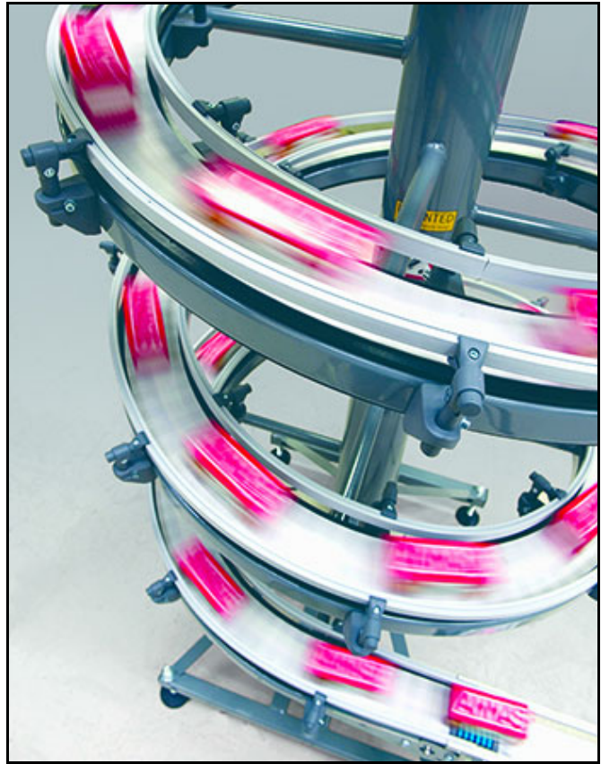
Continuous elevation with spiral elevator
