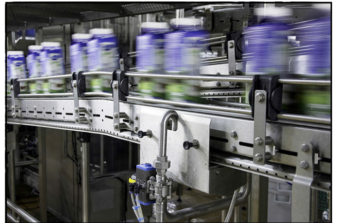
Milk packaging line with Clean-in-Place
