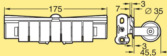
Note. Can only be ordered as a link kit. Roller support items in steel and aluminium. Vertical transportation of cardboard boxes. Link kit 5056654: 1 link + pivot + steel pin.
