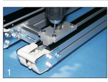
Use a drill fixture to drill two holes at Insert rivets. the end of each slide rail section. Countersink the holes.
