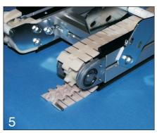
...and remove as many links as necessary to create a light pre-tension in the chain.
