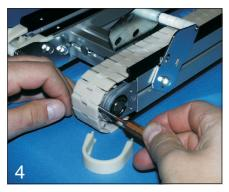
To shorten the chain, use a 2 mm mandrel to press out a steel pin...
