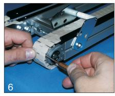
To re-assemble the chain, press the steel pin back to join the links.
