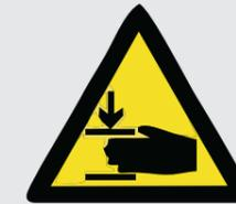
The Pallet locating station could be pressurized, contact of different type than pallets can also activate the lifting / lowering movement. This can cause crush hazard.
