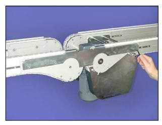
3 Fit the screws (4 x M8) to the inside of the side plates at the driving end
