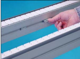
3 Loosen the screws that hold the side cover on the motor side. Use the cross-slotted screw driver. This is done to make attachment of the transfer easy.
