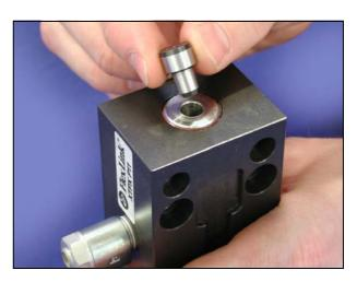
2 Use a soft faced hammer and hit the pin carefully until it reaches the end position.
