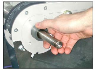
3 Remove the nuts for the slack protection. Use a 10 mm box wrench.
