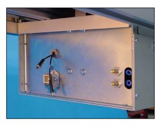
9 Attach the motor cable, the pneumatic tubes and the connections for the sensor cables.
