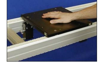
10 Tighten the two locating units to the conveyor beams. Use a set-square to get the pistons in line with the pallet bushings. Use the conveyor beam as a reference.
