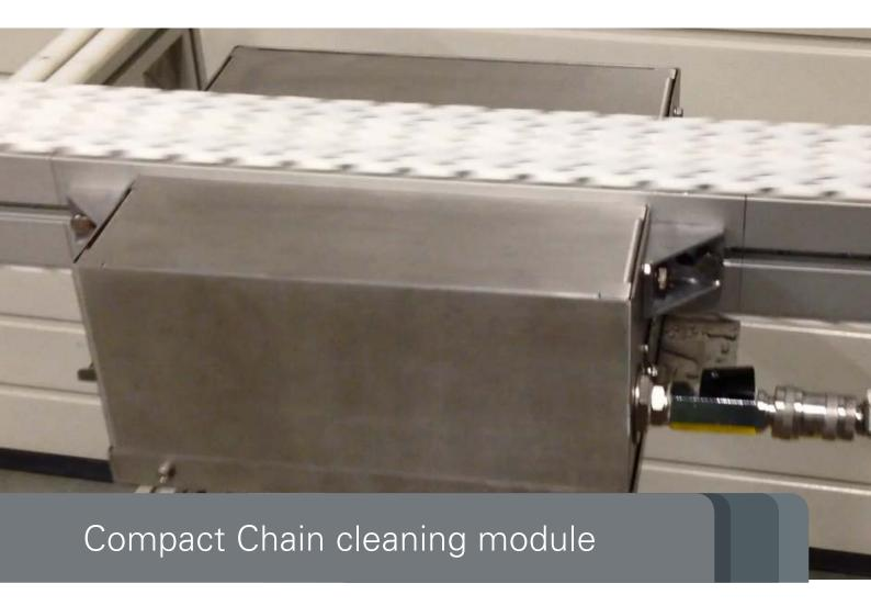
The inline chain cleaning unit is designed to run only when required on a production lines that have product contamination that requires periodical cleaning. The result is a cleaner chain that allows longer production runs without the need for CIP or routine maintenance.
