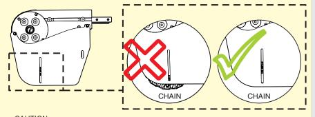
CAUTION The conveyor chain must be maintained during system lifetime. If the conveyor chain is too long, it must be shortened.
