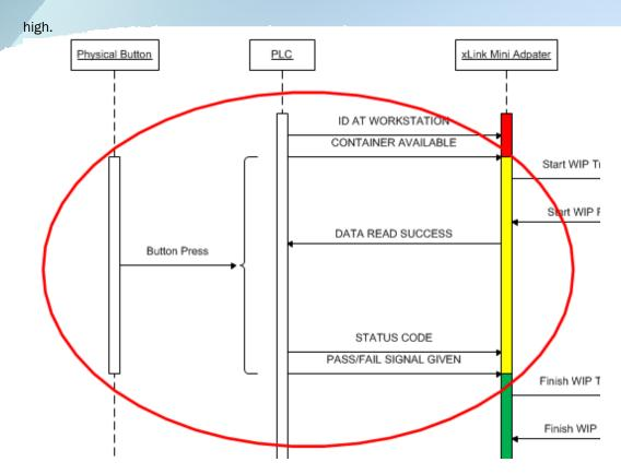
Further, in situations where the status of the PASS / FAIL is determined by Youtilize® (and not by the PLC) the PLC shall ensure the physical button is only enabled when the PASS / FAIL CONTAINER message has been received, and is disabled as soon as the PASS / FAIL SIGNASL GIVEN message is issued.
