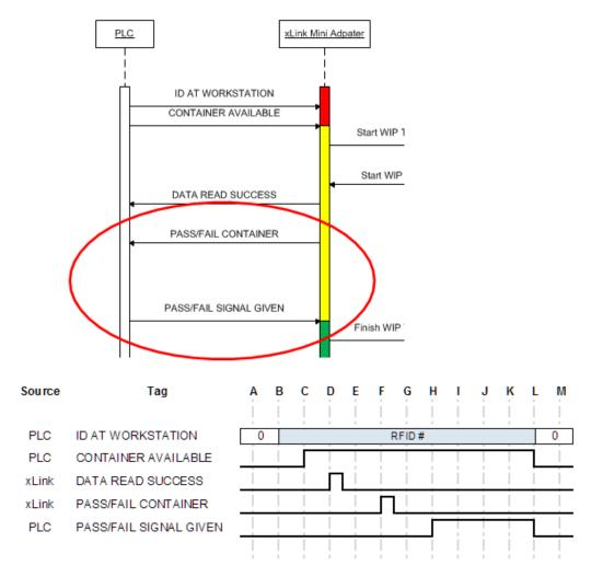
This ensures the same WIP Finish event is triggered no matter which entity determines the Pass/Fail status of the WIP operation.
