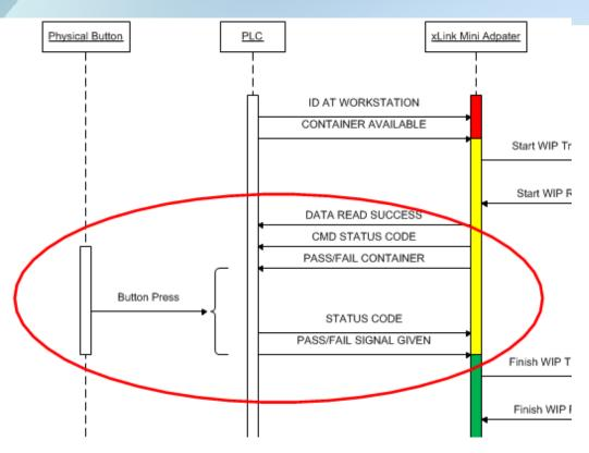
If the Release Button Required status (HS\_WS\_STATUS[Z].6) value is set low then logic within the PLC shall allow the issuing of a Pass/Fail Signal Given without any button press.
