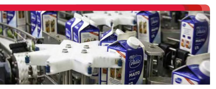
The driven star wheel permits gentle and safe reorientation of bricks.
